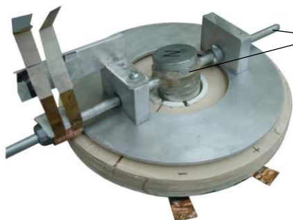
5/16" Round rod Motor Shaft Assembly Magnets and copper pipe commutator will be attached to this rod.
