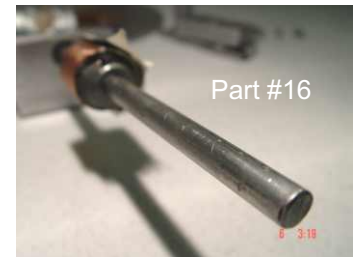
5/16" steel round rod Rotor Shaft
